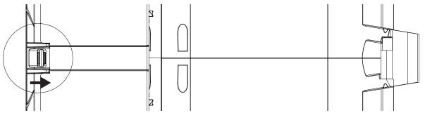
Step 2. Slide the lens tube down into the body until the locking lever can latch. Loosen focus lock knob and adjust focus as desired. Tighten to lock. Reverse process to remove.
