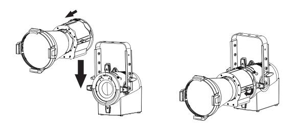
NOTE: Lens tube may need to be moved foward (away from the body) to install or remove. Loosen focus lock knob to adjust.
