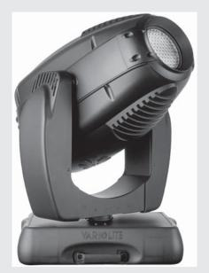
The VARI\*LITE VL3000 Wash luminaire features 6:1 zoomable beam spreader optics, CYM color mixing, variable CTO color temperature correction, a six-position color wheel and separate dimmer and ultra-fast strobe mechanisms. A standard palette of colors is provided with the unit. Custom colors are available.
