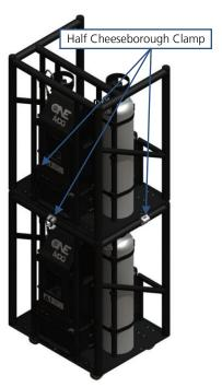
We recommend using **three** T57000 Series Half Cheeseborough from Doughty Engineering with a **Safety Work Load of 750 kg** (1650 lbs) per clamp.
