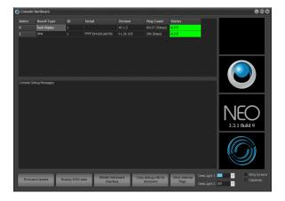
With a monitor attached (sold separately), the Console Hardware display (More > Console Debug Window) will display the firmware version for the Rack Display screen.
