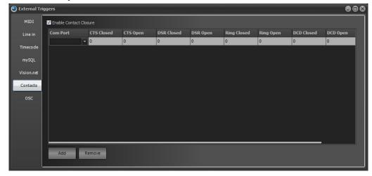
For this wiring we are using the RTS (ready to send) line as the 5V source to complete the closure on the other pins. RTS is set when the COM port is opened and should remain high.
