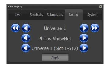
When using the NEO Playback Controller's display to configure the network, the top line is for the DMX universe setting.. This is the same as the Universe column in the System Properties > System I/O Screen on the network table.
