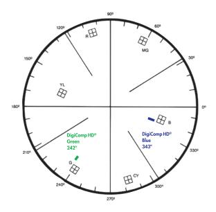
The position of the DigiComp HD Blue and Green signals on the vectorscope indicate the high level of chrominance and luminance that are crucial for a successful matte. The open squares shown on this diagram indicate the points at which chrominance and luminance are maximized. Note that the values of the DigiComp HD colors virtually replicate the theoretical ideals.
