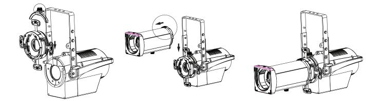
NOTE: Lens tube may need to be moved foward (away from the body) on PLT or internal lenses moved forward on SPX to install or remove. Loosen focus lock knob to adjust.
