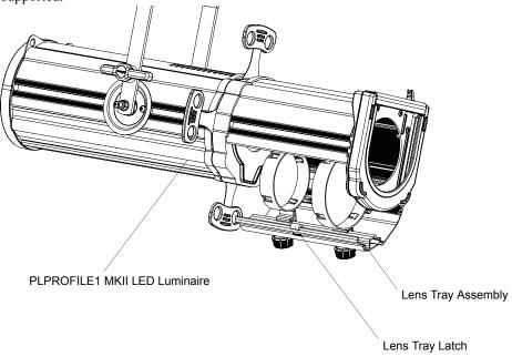
Figure 7: Lens Tray Assembly Removal
