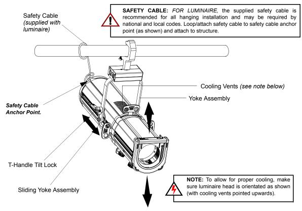
Figure 6: Luminaire Tilt Adjustment
