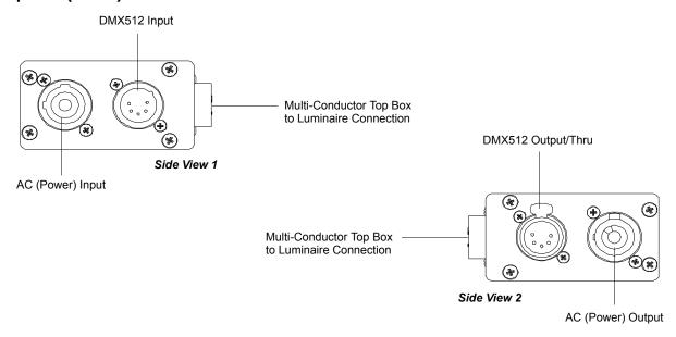
Figure 2: Top Box (PLICB) Connections
