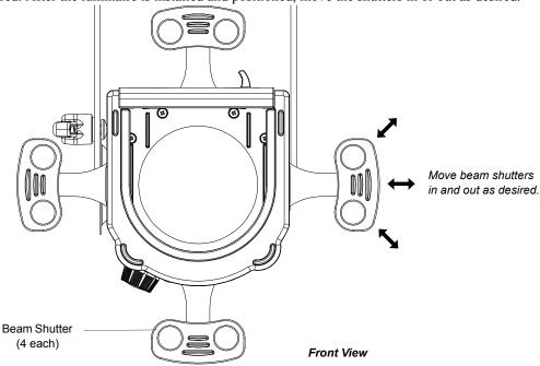
Figure 9: PLPROFILE1 MKII LED Luminaire Beam Shutters
