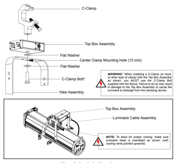
Figure 5: Luminaire Mounting
