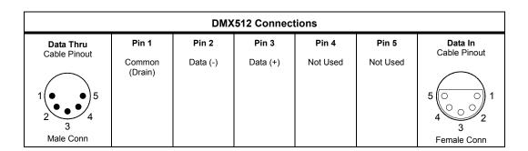
Figure 4: PLPROFILE1 MKII LED Luminaires - DMX512 Connections
