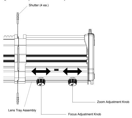
Step 6. Hand-tighten Focus Adjustment Knob to lock position.
