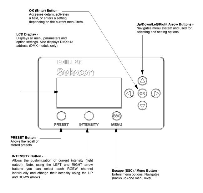
Figure 11: LCD Display and Menu System
