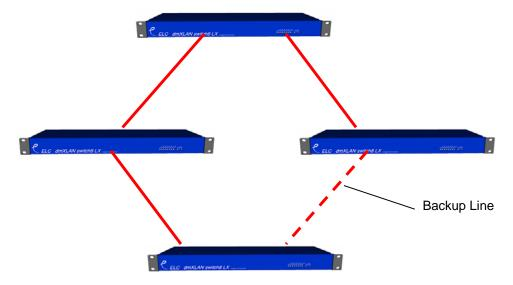
When using standard Ethernet switches, a loop of switches will bring the network down. With the switch8LX ports programmed to loop, the "Backup Line" is detected and automatically disabled. If then during operation (the show) one of the working lines gets broken (or disconnected) all the switch8LX's will then reroute the signal using the backup line, this within 30 to 50 mSec.
