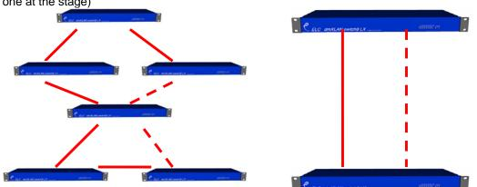
A setup with 2 loops and the smallest setup possible (example 1 switch at the FrontOfHouse and one at the stage)
