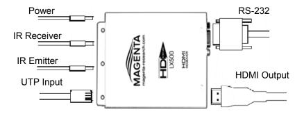
Figure 3-2. Connections on the Receiver
