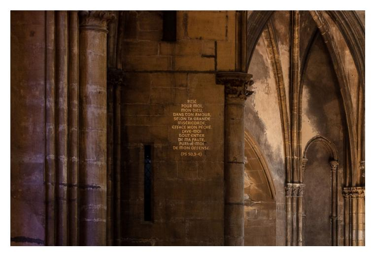
Designers at Nouvelle Étiquette explained that "the key to the success of this installation was to control the intensity of the projections while preserving the legibility of the texts." The 3000K Image Spot fixtures met this requirement by creating gobo projections in warm light without compromising the sharpness of the projected textual image.
