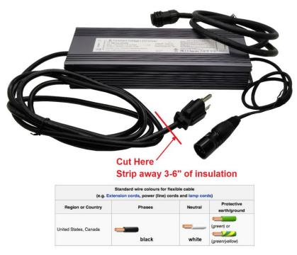
If you wish to use bare wire input, cut the cable close the Edison connector and remove the connector. Strip away 3-6" of the black insulation, careful not to damage the insulation on the interior wires. The black wire is the Line (L), the white wire is Neutral (N), and the green wire is Ground (G). Please take careful note of the Input specifications printed on the PP36, and confirm that you are wiring it to compatible power source.
