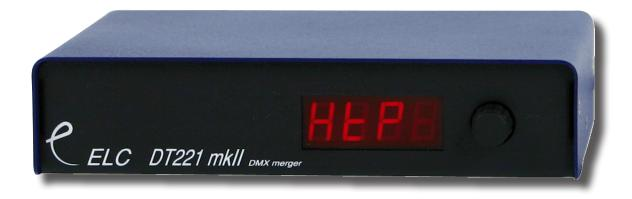
The DT221 MkII is a desktop or truss mounted DMX merger that combines 2 DMX sources into one single DMX source using either HTP, LTP or priority (DMX-A has priority unless it fails, then DMX-B is output).
