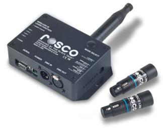
An additional receiver option includes the use of a 2nd CubeConnect<sup>™</sup> Transceiver, allowing CubeConnect<sup>™</sup> to be deployed with any product which accepts DMX or to convert existing non-data track systems into intelligent systems.
