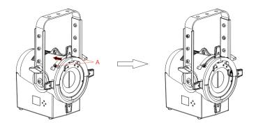
Step 1. Loosen the two screws at A and move the shading plate backward. Tighten the two screws.
