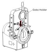
Step 2. Snap the gobo holder into the luminaire.
