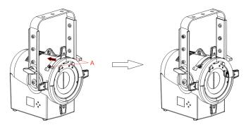
Step 1. Loosen the two screws at A and move the shading plate backward Tighten the two screws to fix it.
