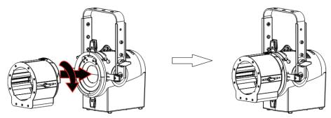
Step 2. Insert the lens tube into the adapter. After achieving the desired beam edge, tighten the locking bolt.
