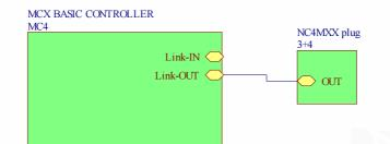
During operation, the NC4MXX plug must be connected to the last controller in chain
