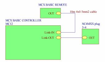
During operation, the NC4MXX plug must be connected to the last controller in chain
