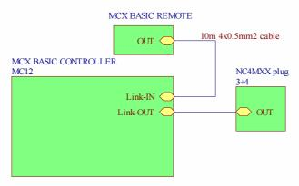
During operation, the NC4MXX plug must be connected to the last controller in chain
