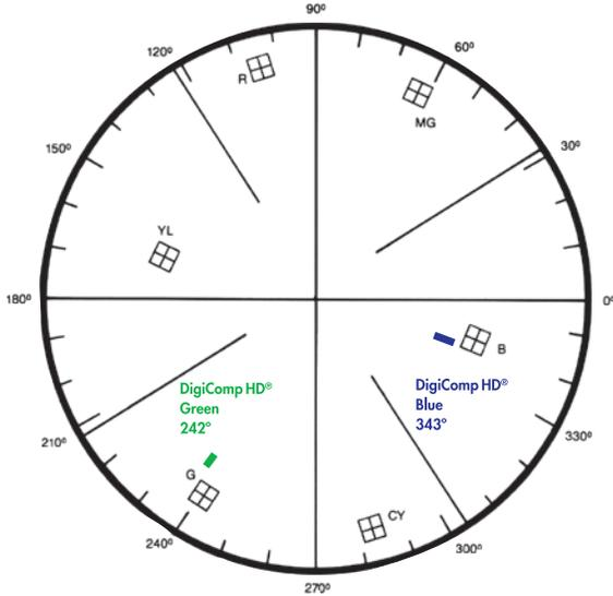
The position of the DigiComp HD Blue and Green signals on the vectorscope indicate the high level of chrominance and luminance that are crucial for a successful matte. The open squares shown on this diagram indicate the points at which chrominance and luminance are maximized. Note that the values of the DigiComp HD colors virtually replicate the theoretical ideals.
