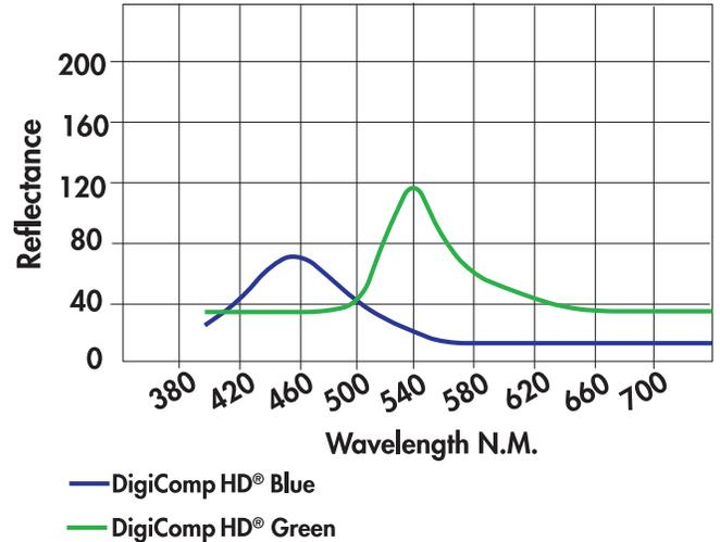
The graph shows where the DigiComp HD Blue and Green colors fall on the spectrum and the percentage of the wavelength (color) that is reflected back to the viewer/camera.
